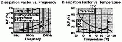
Capacitors used for coupling small signals between stages, in active filters, the shunt caps on crystal filters, or in the transmitter output filter, should
