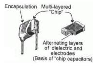
capacitances in physically smaller packages. Their characteristics are very similar to disk ceramics. They are encapsulated in epoxy to withstand insertion, soldering and solvent cleaning by the automatic PCB
