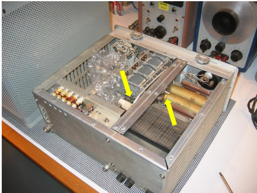
Figure 3. First surprise – No tubes. I forgot that Mister Thorough removed the tubes and padded the plate clips and braid before moving....Hmmmmmm, Time Out! ... and it is tube hunting time. With the current cost of 811As, read that PANIC time!
