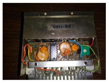
This appears to be a modification dating back to the 1970's and was designed to improve the relatively poor large-signal handling characteristics of the early models of the FT-101. The IC is a double balanced mixer (in this case a LM1496) and is wired to replace the 3SK39/3SK40 FET used as the Rx 2<sup>nd</sup> mixer.
