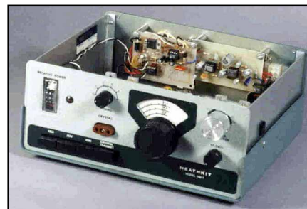
An interior view of the HW-7. The audio filter is on the right-hand side of the rear panel and the NoGa PiG is piggybacked on the left side of the rear panel.
