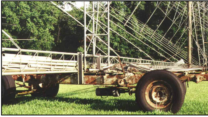
The 1947 Ford pickup chassis and 1/3 horsepower dc motor that rotates the MBA.
