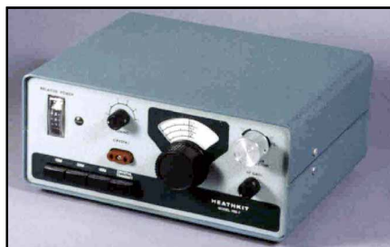
An exterior shot of the HW-7. Note the large aluminum knob on the preselector shaft. This knob provides extra mass (weight) and the added circumference makes it easier to accurately peak the RF front end on the HW-7.
