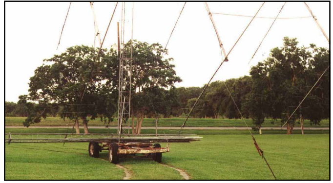
Here you can clearly see the concrete tracks as well as the cable tie-down that secures the MBA when it is not in use.
