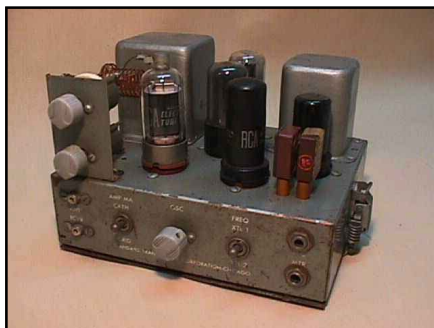
The Stancor ST-203-A with the cover removed.
