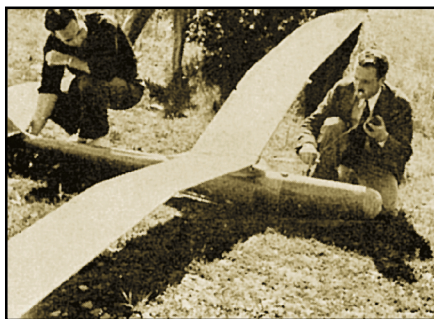
Hull (right) and his model soaring plane at the Elmira soaring meet in the summer of 1938. The plane is a gull-wing with a 16-foot span. It had been equipped with radio control by Hull and Bourne, W1ANA, the latter acting as control operator in flight.
