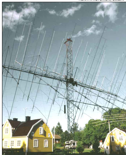
The SM5FRH 2-meter EME array in Katrineholm, Sweden.
